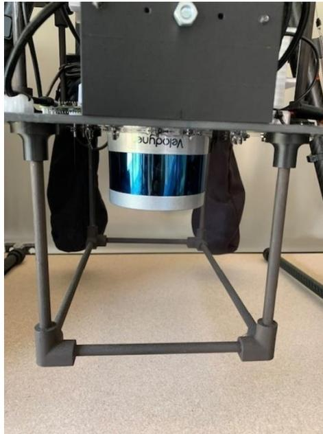
Figure 12 Velodyne LIDAR Installed in a Cage on Matrice 600 Pro
