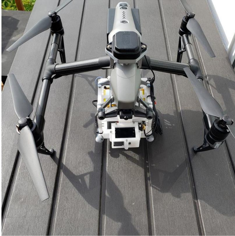
Figure 57 Sensor Enclosure Attached to a DJI Inspire Pro 2
